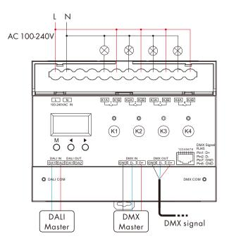
Note: The maximum surge current of the AC output is 120A, the sum of surge current of multiple resistivel load or inductive load (LED drivers )should not exceed its maximum value.
