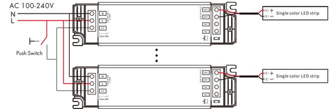
The provided AC Push-Dim interface allows for a simple dimming method using commercially available non-latching (momentary) wall switches.
