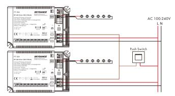
The provided AC Push-Dim interface allows for a simple dimming method using commercially available non-latching (momentary) wall switchs.
