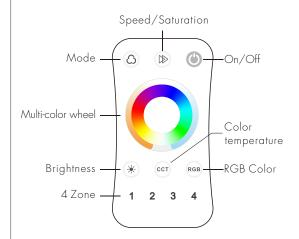
R8-5 can also be used as four zone universal remote, each zone can match single color, dual color(WW/CW), RGB, RGBW or RGB+WW/CW controller.
