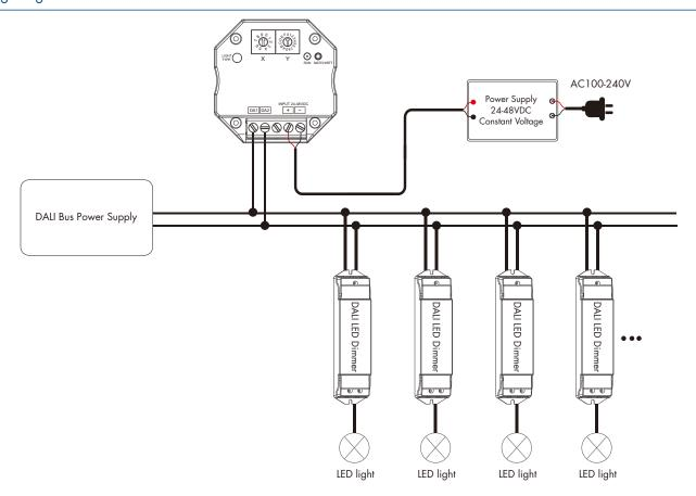
Note: When DA-M(WT) is working, because the power consumption of the WiFi module is too large, it cannot be powered by the DALI bus power supply.
