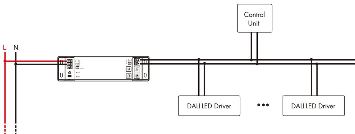
**DALI LED driver:** include DALI dimming controller, DALI dimming driver, etc.
