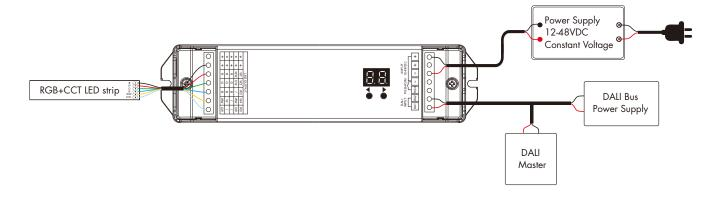
Note: It is not recommended to use both the DALI master and the self-resetting switch for dimming control.
