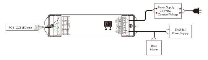
Note: It is not recommended to use both the DALI master and the self-resetting switch for dimming control.
