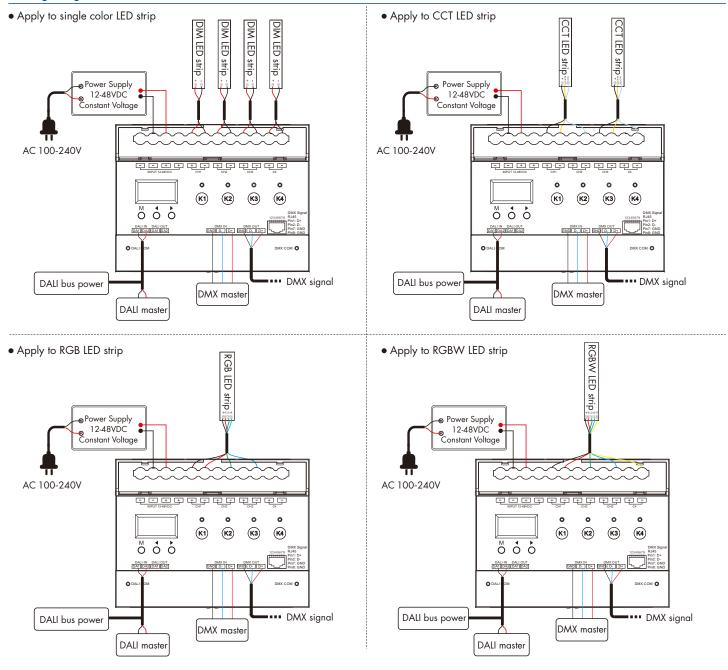
Note: The dimmer can't input DALI signal and DMX signal at the same time, you can only select one of the control methods.
