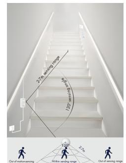
The stair light application requires a set of sensor dimming controller on each side of the stairs, both up and down.
