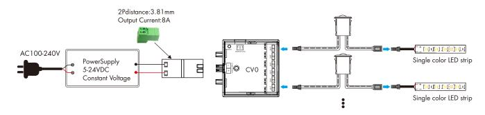
• Power supply using cabinet constant voltage power supply + junction box
