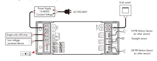
Note: The W2 channel output is not dimmable and is used for inductive control of other low voltage powered devices.
