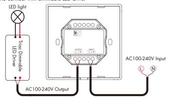
Note: When calculating the maximum number of load lamps or drivers, the input power or input current parameters of a single lamp or driver must be used, the output power parameters can not be used.
