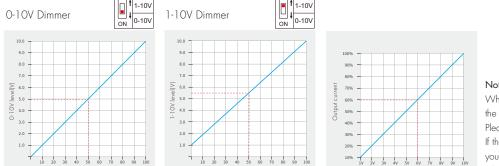
When the output channel is off, the output dimming signal is OV or 1V. Please read the dimming section of the dimming driver manual. If the dimming characteristic curve is the same as left, you must select 1-10V dimmer and use AC OUT function, otherwise you can't turn off the lights.
