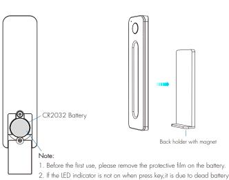
It the LED indicator is not on when press key, it is due to dead battery or bad contact caused by multiple plugging, please replace the battery, or raise the battery shrapnel with a screw driver.
