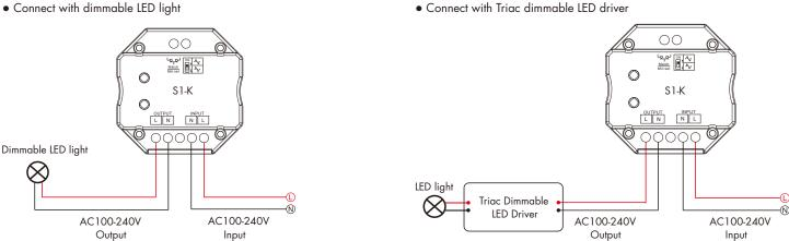
Note: When calculating the maximum number of load lamps or drivers, the input power or input current parameters of a single lamp or driver must be used, the output power parameters can not be used.
