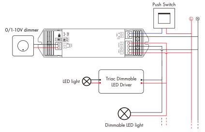
Note: When calculating the maximum number of load lamps or drivers, the input power or input current parameters of a single lamp or driver must be used, the output power parameters can not be used.
