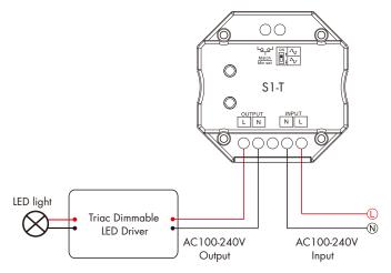
Note: When calculating the maximum number of load lamps or drivers, the input power or input current parameters of a single lamp or driver must be used, the output power parameters can not be used.
