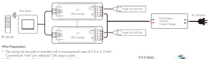
2. When wiring is installed, the terminals must be tightened. If they are not tightened, the contact point resistance will be too high and the terminals will easily burn due to heat when used at full load for a long time.
