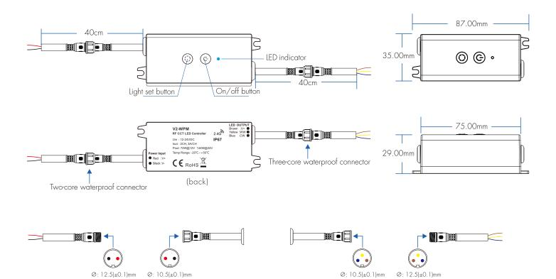
NOTE: When installing, align the insert and tighten the nut.
