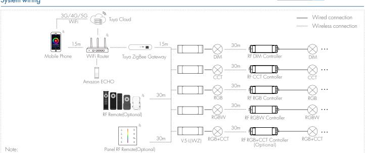
1. The above distance is measured in spacious (no obstacle) environment, please refer to the actual test distance before installation
